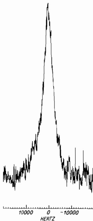
Fig. 3. ^{99}\text{Tc} NMR spectrum of \text{Tc}(\text{CO})_3\text{Cl}(\text{PPh}_3)_2 ( \delta = -1488 \pm 1 ppm vs. \text{TcO}_4^- ). Number of scans 324, Lorentzian folding with 100 Hz, 7.6 Hz/point.
